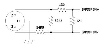
Resistors can be either 1% thick film (0603 or 0805) or RN55 thru hole types.
