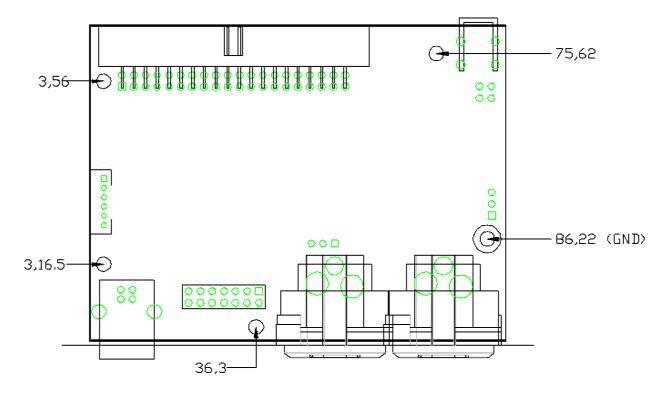
Holes are 3.2mm suitable for 4-40 or M3 Screws
